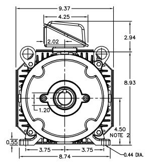
NOTE 1: C-FACE & TACHOMETER MOUNTING 1/2-13 TAP, 1.00 DEEP, ON A 7.25 DIA. BOLT CIRCLE FACE RUNOUT AND ECCENTRICITY 0.004 MAX. T.I.R.
