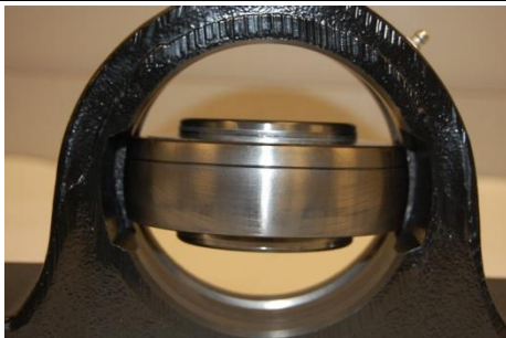
Figure 3) Loading bearing into loading slots
