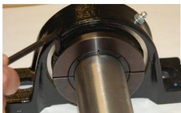
Figure 1) Set screw tightening on a Centrik-Lok bearing
