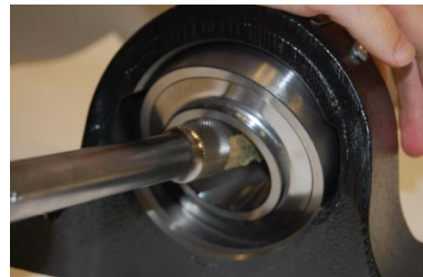
Figure 4) Torquing bearing 90° into housing
