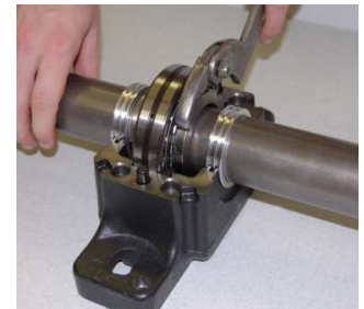
Figure 2) Tighten Until Snug
