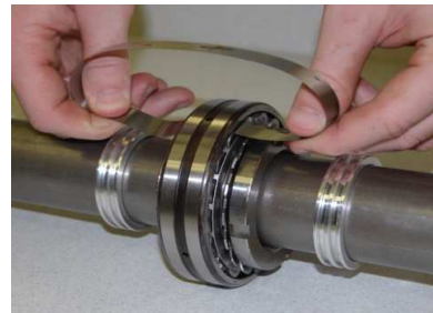
Figure 1) Measuring Initial Clearance
