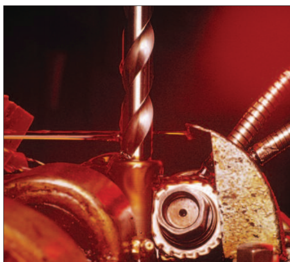
Flute milling of large diameter twist drills
