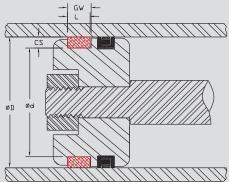
Part numbers call out ØD and L and will only call out the CS if it does not equal 0.125" Example: WR-1750x500 is a 1.750" OD x 0.500" L
