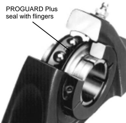
On SXR bearings, optional flingers can be added to form a tight labyrinth with the PROGUARD Seal and provide additional seal protection against contaminants and debris.
