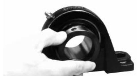
The inner ring of the bearing is locked to the shaft by a quarter-turn of the eccentric collar in the direction of shaft rotation. The collar is secured in place with a single setscrew.
