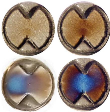
Figure (4) Acceptable Changes in OSS. In most cases change will be between top 2 pictures
