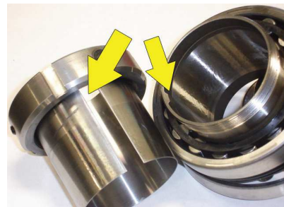
Figure (2) If sleeve is removed from inner ring, align spline with slot in sleeve to reinstall.
