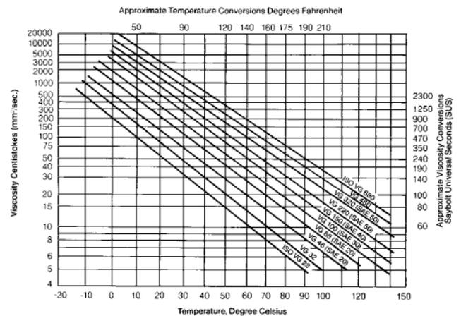
Figure 2 Viscosity-Temperature Chart
