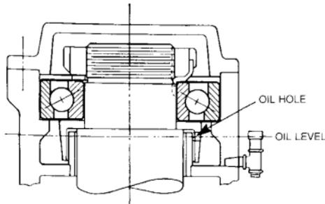
The design above is suited for uni-directional thrust. If reversing thrust is present, it must be taken by an opposed bearing mounted at the bottom of the shaft. Note that the oil is lifted into the bearing by means of the inverted rotating cone. Attention is called to the drilled hole which prevents possible siphoning out of the oil when the shaft is stationary.
