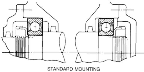
This is the ideal mounting for a shaft supported by two ball bearings, and has these advantages:
