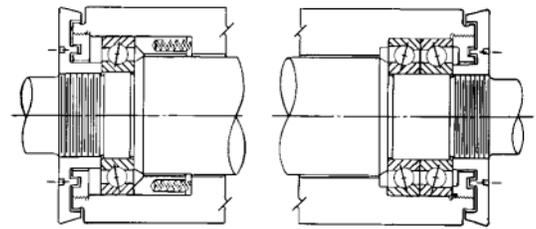
In this arrangement the shaft is supported at the right end by a duplex pair mounted in the back-to-back relationship. These bearings may be supplied as a preloaded set if operating conditions require that deflections be minimized. The bearing on the left end of the shaft is a single-row deep-groove bearing which floats axially in the housing and is lightly spring loaded to remove residual clearances.
