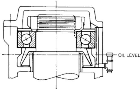
The sketch above shows the conventional method of circulating oil in a vertical application. Note that the dish-shaped oil thrower pumps the oil up through the drilled hole in the housing from which the oil flows downward through the bearing by gravity. Reverse thrust loads must be carried by an opposed bearing.
