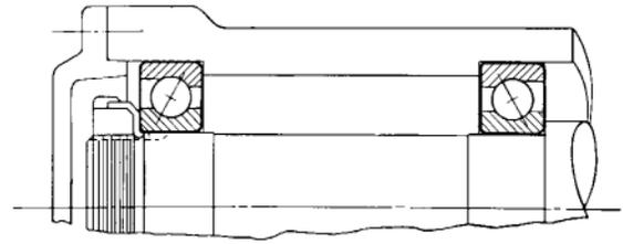
This construction requires housing shoulders, and a lock nut on the shaft. Adjustment is made by means of the lock nut. The left hand bearing should have a sliding fit on the shaft.
