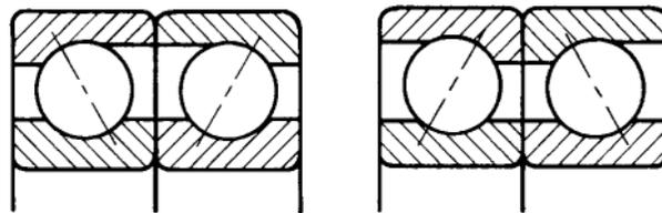
Figure 4 Angular contact ball bearings pair mounting arrangements.
