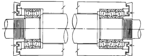
The shaft is located axially by the arrangement on the right end of the shaft which consists of a pair of tandem bearings opposed back-to-back against a single bearing. The duplex back-to-back pair on the left end of the shaft is free to move axially in the housing. This mounting arrangement has great rigidity.
