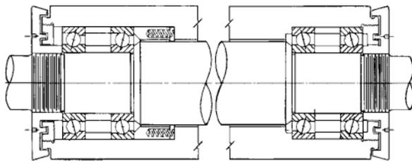
In this arrangement, the duplex tandem pair on the left end of the shaft is spring preloaded against another duplex tandem pair on the right. The pairs at either end are separated by equal length spacers between bearing outer rings and inner rings. This arrangement produces good shaft rigidity due to the multiple shaft support.
