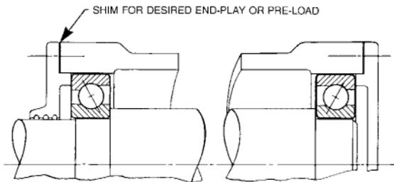
This construction requires a shoulder on the shaft, and a clamping member of the outer ring, with shim adjustment.
